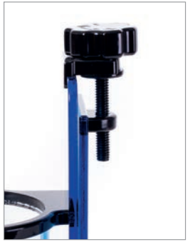
Install the inside plate with the collection cup holder onto the other inside plate.
